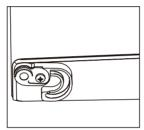
5. Unscrew the bottom hinge, and remove the adjustable foot from the left side to the right side.
