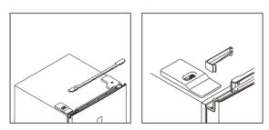
2. Unscrew right top hinge cover, and disconnect connectors of door switch and display.
