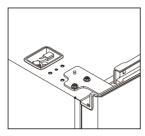
12. Connect connectors of door switch and display, and install the left top hinge cover.
