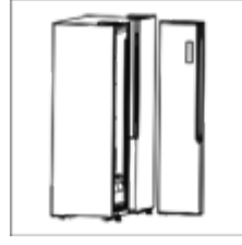
4. Lift the door and place it on a soft pad. Remove the other door using the same process.
