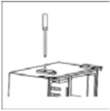
1. Unscrew hinge cover using a Philips screwdriver.
